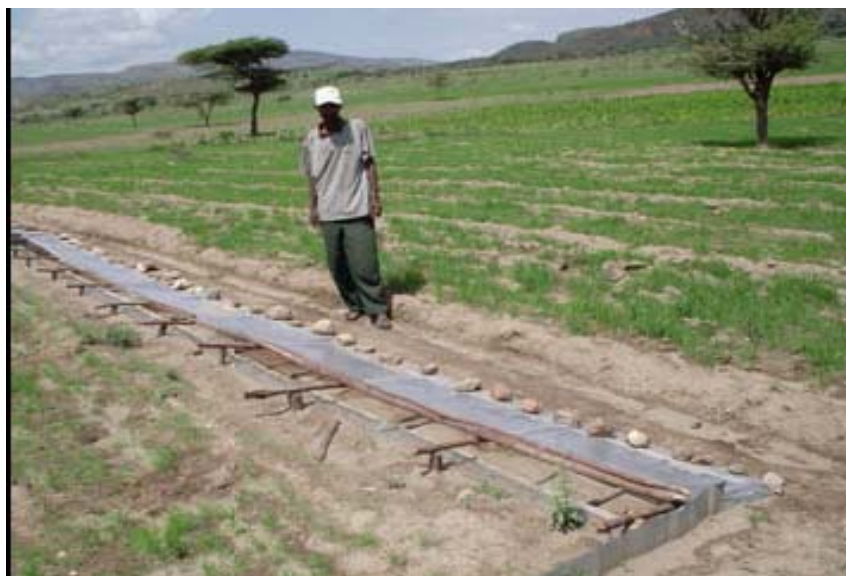
Figure 6.2. Runoff collecting trough installed at the bottom of a 10 m x 10 m plot.
