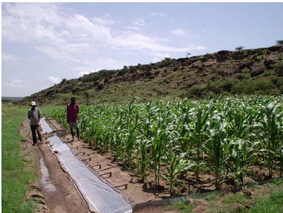
Figure 5.1. Surface runoff collecting trough covered with hanging plastic sheets to prevent direct precipitation.
