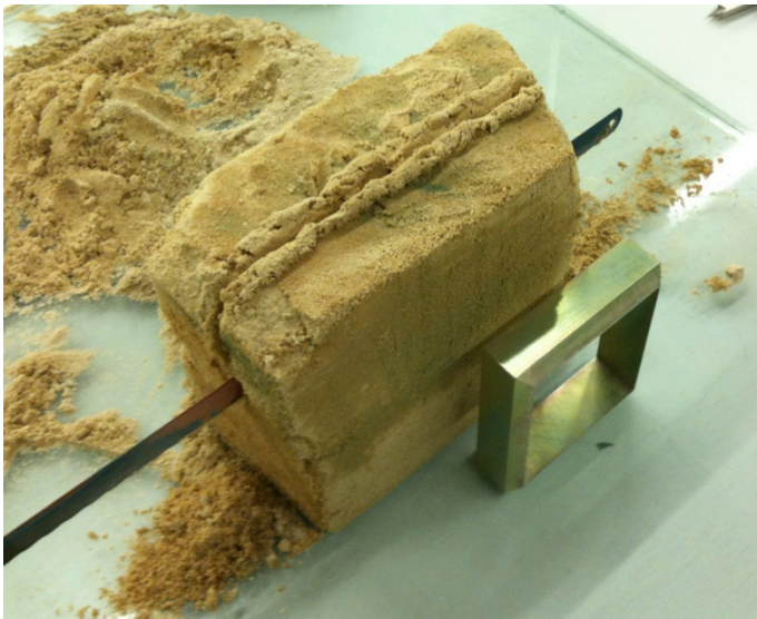
Figure 10: Sawing a slice of calcarenite by using a hacksaw blade [personal photograph, 2013].
