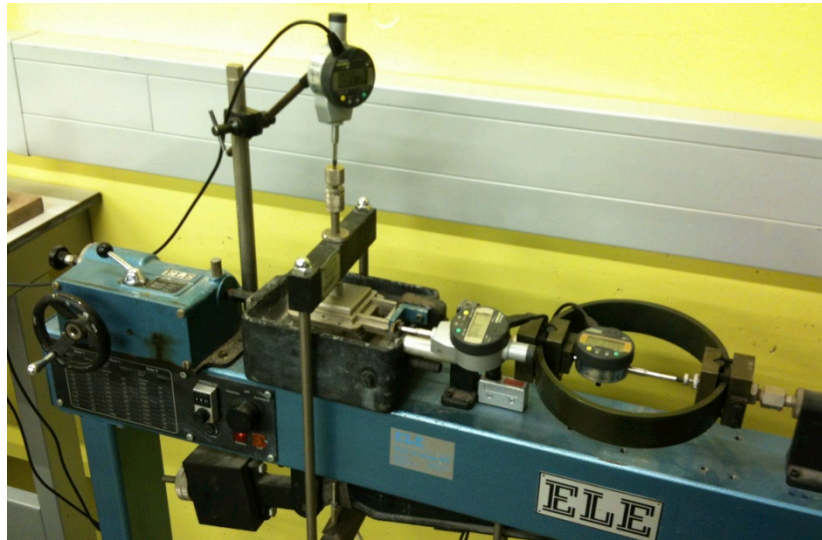
Figure 13: The shear box test apparatus, with the loaded sample in the black container, and all indicators installed [personal photograph, 2013].
