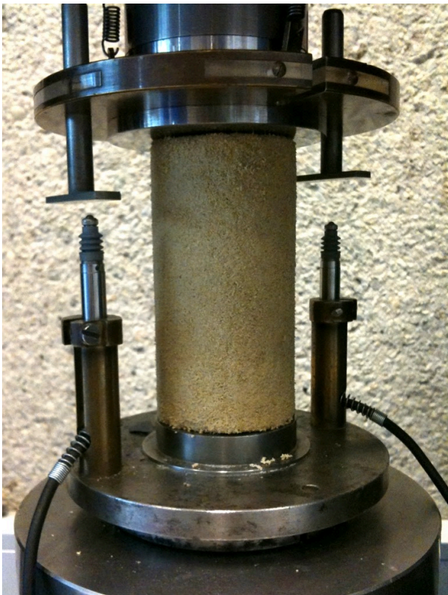
Figure 8: Sample ready for unconfined compression test (with vertical displacement indicators not positioned yet) [personal photograph, 2013].
