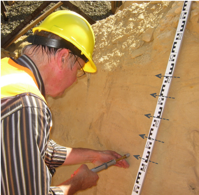
Figure 7: The spring-loaded pocket penetrometer being used by W. Verwaal [personal photograph, 2013]. The arrows point out rows where penetrations were performed (tiny holes are hardly visible).
