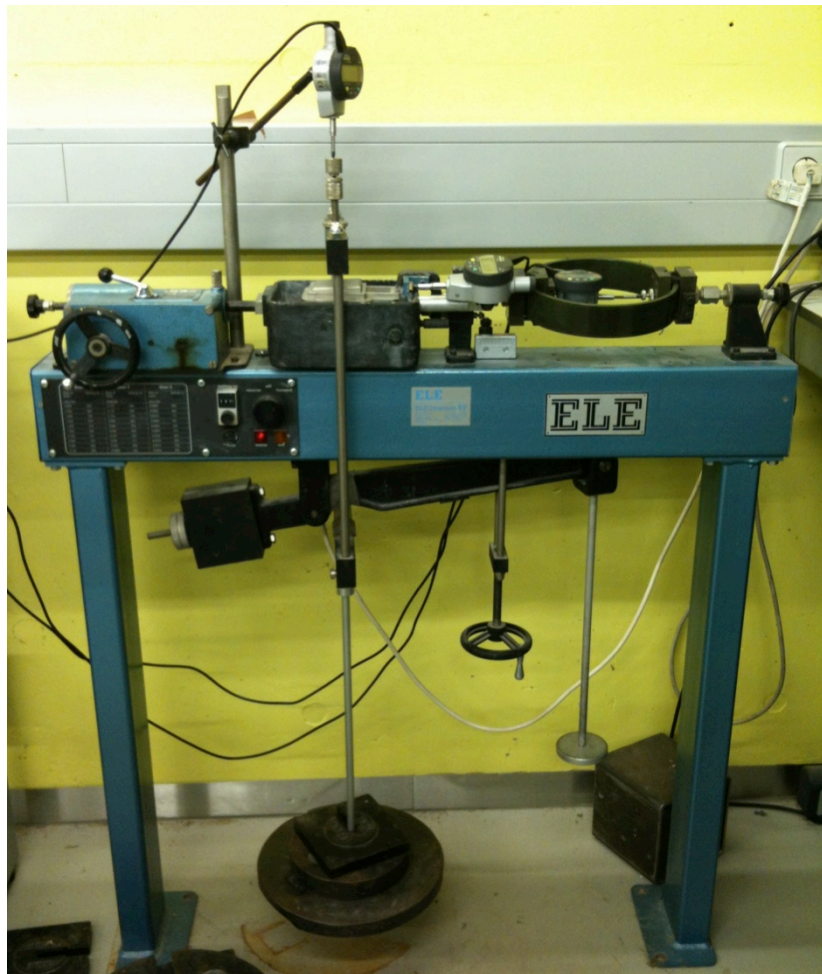
Figure 14: Overview of the complete shear box test apparatus, including load hanger with load [personal photograph, 2013].
