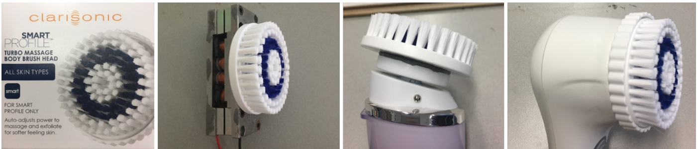
Fig.68 Overview of the brush and the brush attached to the different products/actuators used to generate the motion
