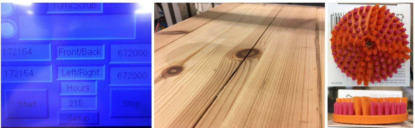
Fig.98 Overview of the running time of the test (left), the damage caused on the floor (centre) and the damage on the brush (right)
