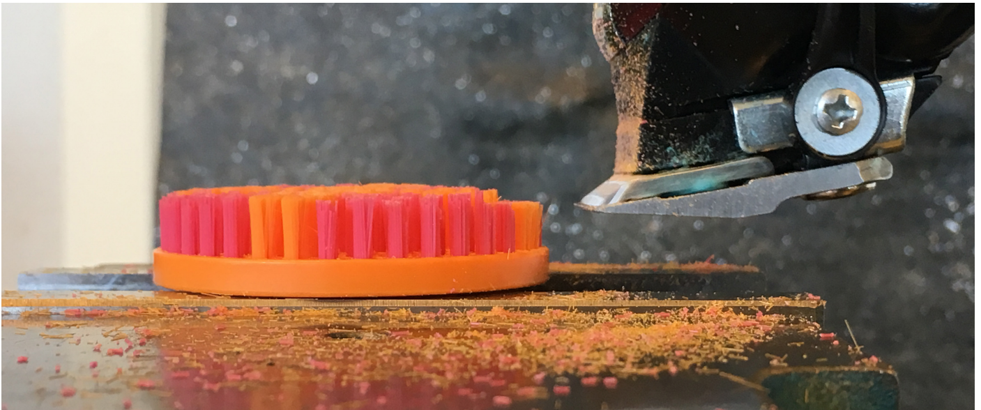
Fig. 110 Close up view of the bristles being cut down using a razor attached to a CNC machine
