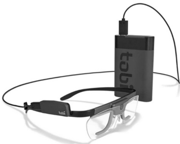
Fig. 161 Close up view of the different components of Tobii Pro Glasses 2. The glasses on (Right) and the software (Left)
