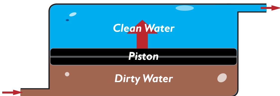
Fig.28 Diagram of syringe principle water tank.
