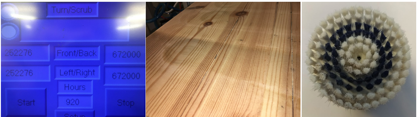
Fig.97 Overview of the running time of the test (left), the damage caused on the floor (centre) and the damage on the brush (right)
