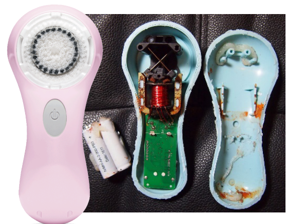
Fig.67 Overview and inside view of Clarisonic Mia 2
