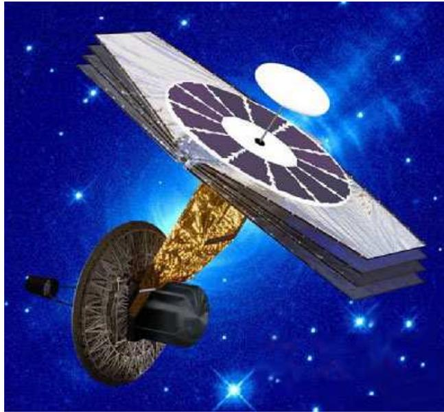
Figure 1.19 A SAFIR concept based on the segmented-mirror technology to be employed for the JWST [Official website]
