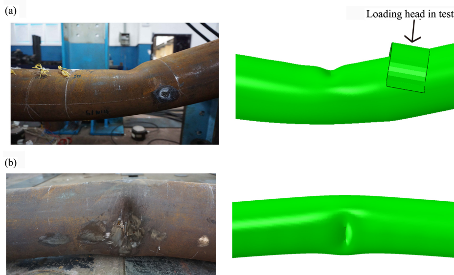
Figure 5.5: Representative failure mode of specimens: (a) specimen without damage (S1N4); (b) specimen with metal loss on its compression side (S3N3).
