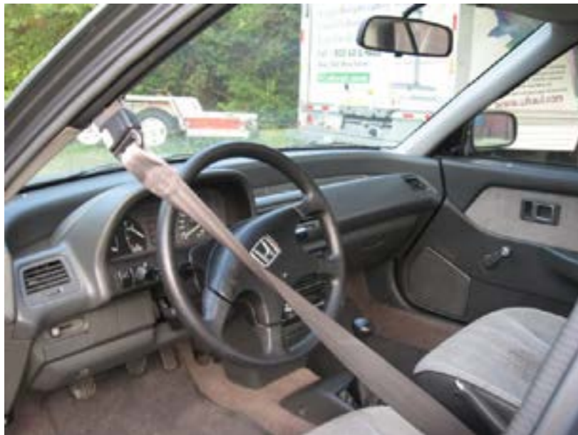
Figure 12: Automatic seatbelt (Orlove, 2017)
