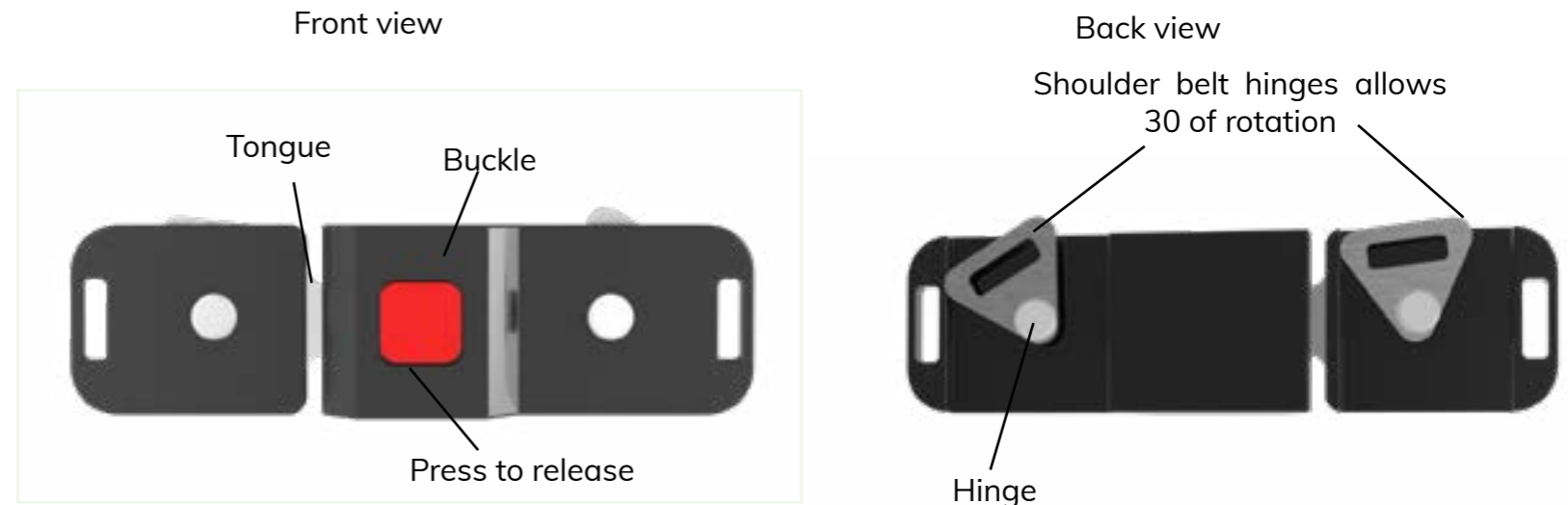
Fig 52 : Central release buckle
