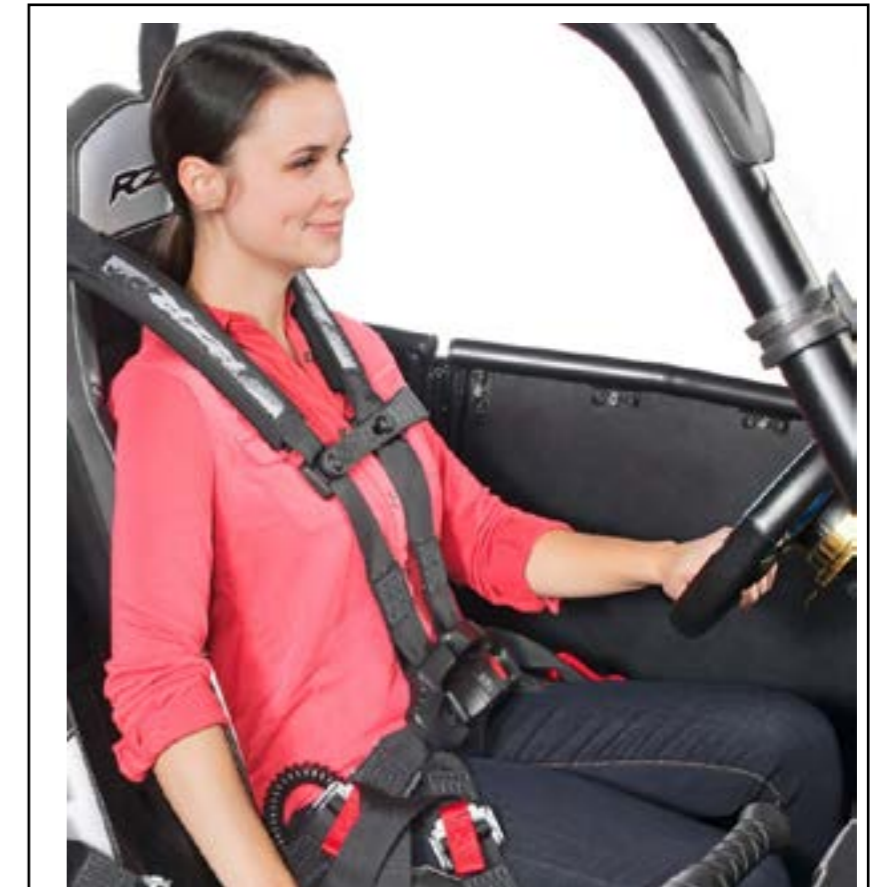
Figure 32 : Contact points for four point belt
