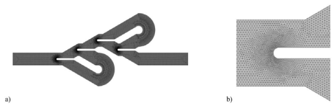
Figure 3. (a) Overview and (b) refined mesh near the divider baffle for the computational domain.
