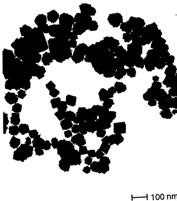
Fig. 5 TEM micrograph of TiN powder, typical for synthesis experiments within the temperature range 923–1173 K
