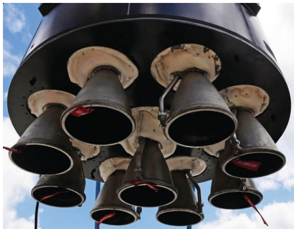
Figure 3.2: Electrons first stage engine configuration featuring 9 Rutherford engines [2]
