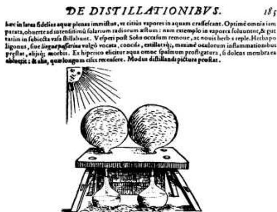
Figure 1.1 – Della Porta distillation apparatus published in Magiae Naturallis (1558).
