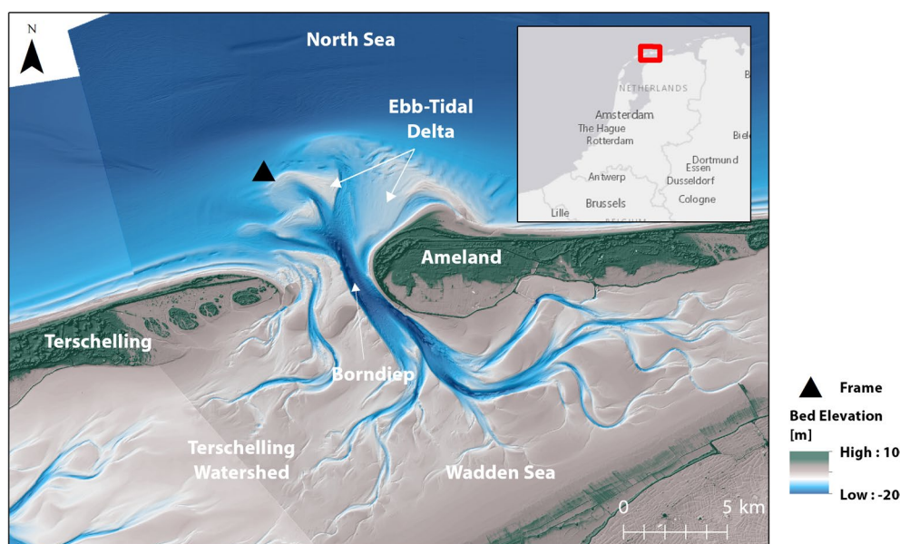
Figure 2. Overview of measurements during the September 2017 field measurement campaign at Ameland Inlet, including the frame (AZG-F4) bearing the instruments used in this study. Bathymetry source: Rijkswaterstaat Vaklodgingen. Elevation source: Actueel Hoogtebestand Nederland (AHN), Rijkswaterstaat. Basemap sources: Esri, HERE, Garmin, ©OpenStreetMap contributors, and the GIS user community.
