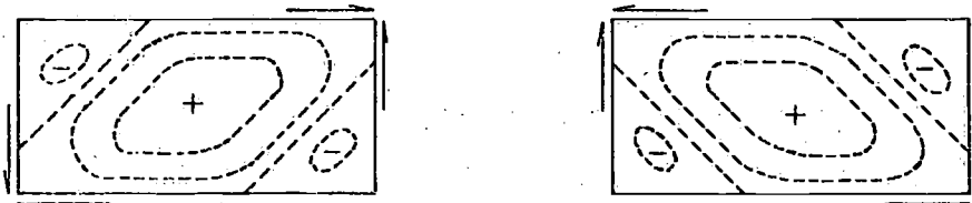
Figure 2. Deformations due to equal but opposite buckling loads, /5/.
