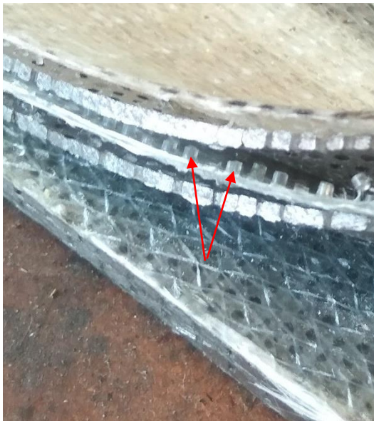
Figure A.o.1: Resin Micro-Structures Forming Through the Perforations in the Steel
