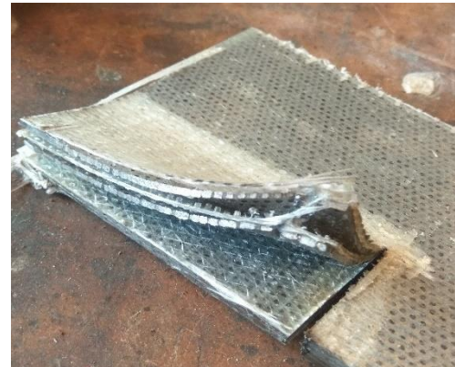
Figure A.0.6: Material Damaged by Inappropriate Saw
