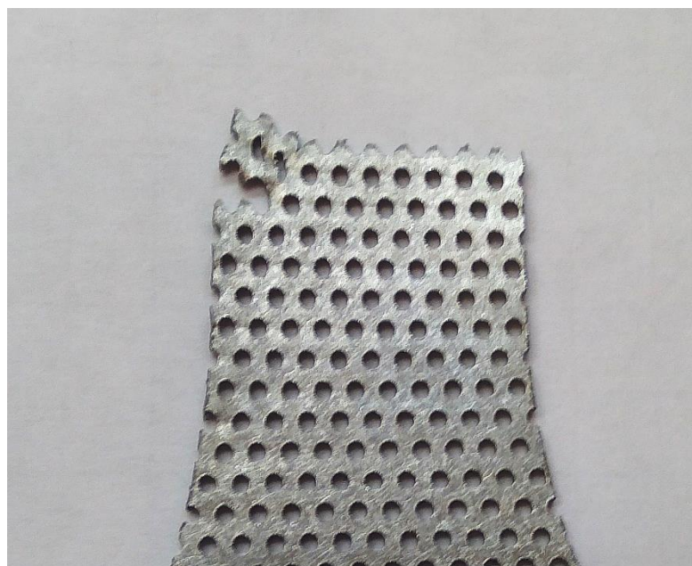
Figure 3.9: Failed Perforated Steel Sample
