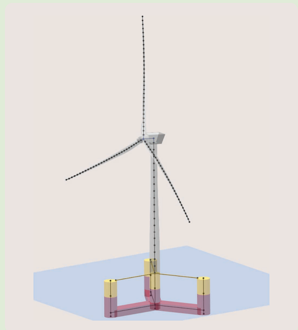
FIGURE S5 A representation of a floating wind turbine with beam elements connected in a multibody formulation.
