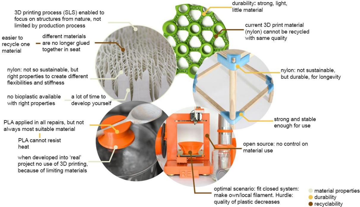
Figure 15. annotations related to the material input of additive manufacturing
