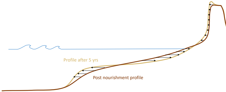
Figure 2.14.: Schematic view of observed cross-shore behavior at the Hondsbossche Dunes nourishment including an increase in dune volume and equilibration of beach width, modified from Elko and Wang (2007).
