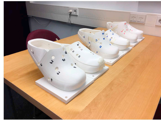
Fig. 3. The three pairs of 3D printed foot shells.
