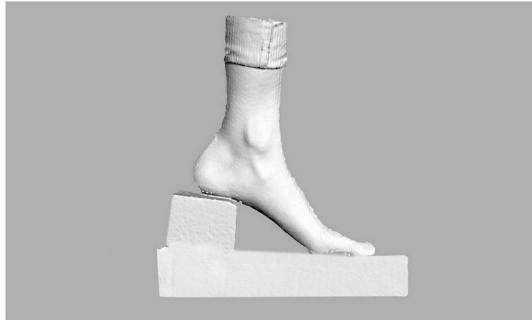
Fig. 2. Example of 3D scan in toe-off position, obtained by placing a block of polystyrene 65 mm high under the participant's heel.
