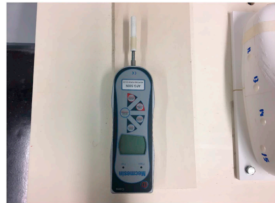
Fig. 4. Mecmesin AFG 500N with the 3D printed rod screwed on top.
