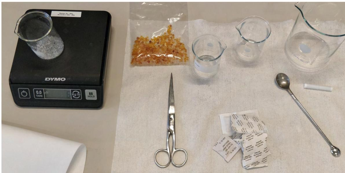
Figure D.1: Overview of required components to make a  $\text{NaOH} + \text{Na}_2\text{SiO}_3$  solution with DIY  $\text{Na}_2\text{SiO}_3$ .
