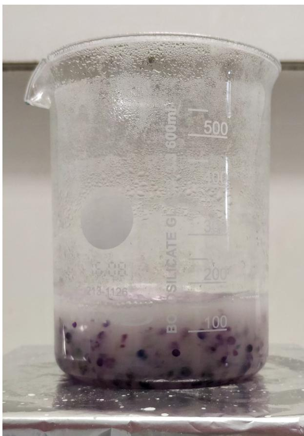
(a) Dissolving silica gel in a  $\text{NaOH}$  solution to create  $\text{Na}_2\text{SiO}_3$ .
