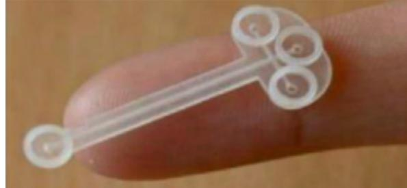
(b) Lab-on-a-chip for capillary gel electrophoresis made using a structural and support material ink. Adopted from [52]
