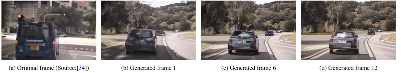
Figure 1. Augmenting scene in Prescan [37], the new scene is mapped to the photorealstic domain using the video diffusion model. Car in front is idle while the car in the back of the scene is driving away.
