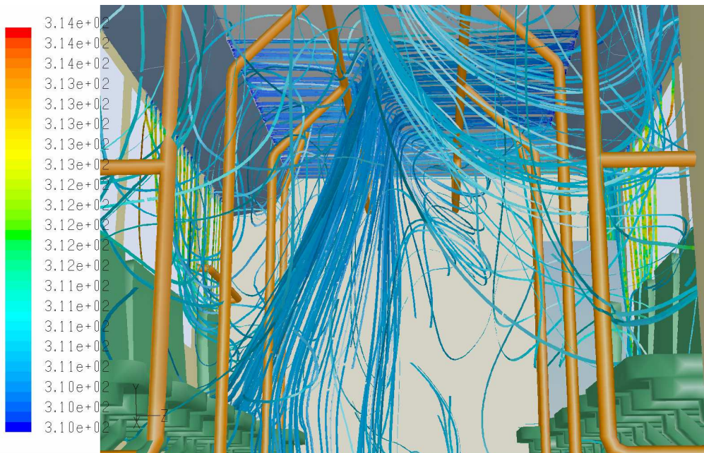
Path Lines Colored by Static Temperature (k) (Time=2.0000e+02) May 12, 2006 FLUENT 6.1 (3d, segregated, S-A, unsteady)
