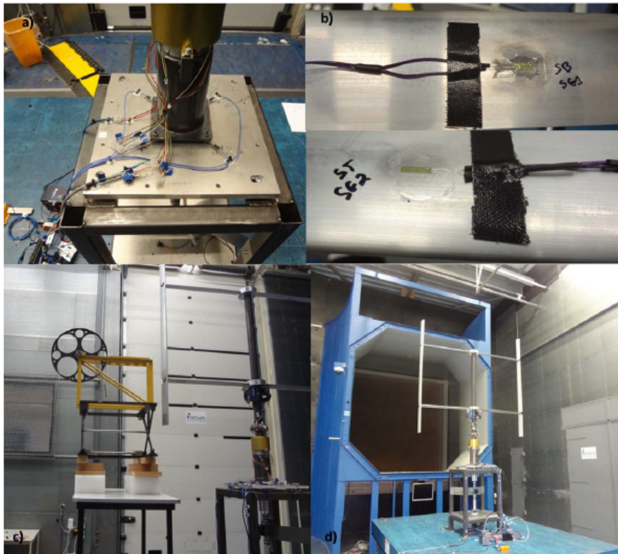
Figure 1. Experimental setup for PitchVAWT in the Open Jet Facility wind tunnel at TU Delft. Thrust is measured through load cells between the main bearing housing and the base mounting plate (top left image).
