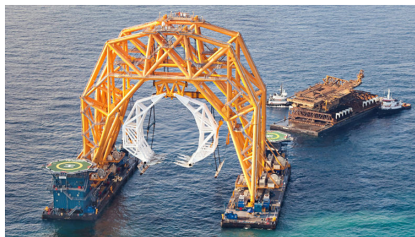
Figure 6.28: Versabar 10.000 ton lifting capacity [78]
