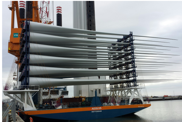
Figure 5.6: Blade rack on the Aeolus jack up vessel [W32]
