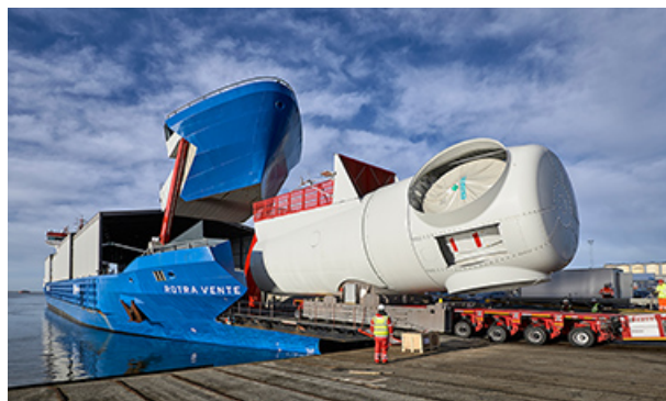
Figure 7.10: Siemens customised turbine transport vessel in Esbjerg [W30]
