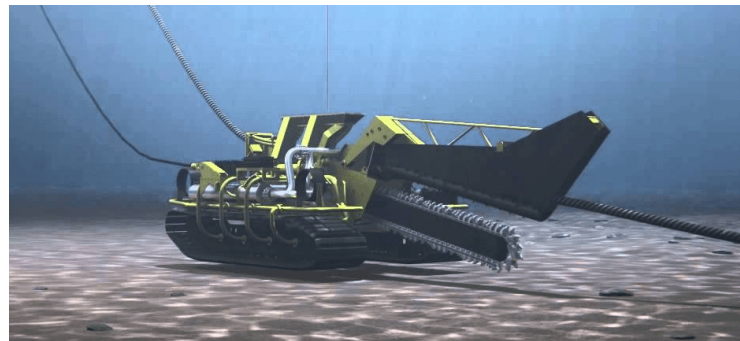
(b) Trench machine [W33]
