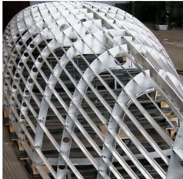
(a) Ship construction without outer plate [W12]
