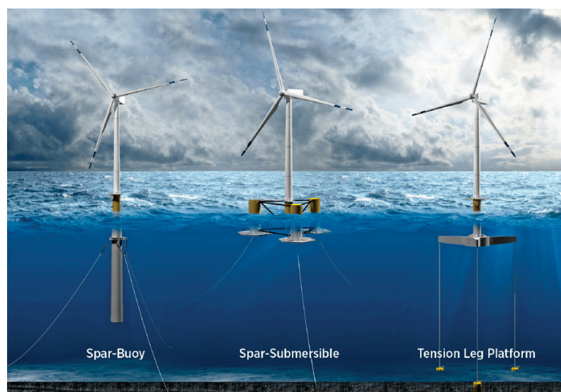
Figure B.2: Main floating foundation concepts [69]
