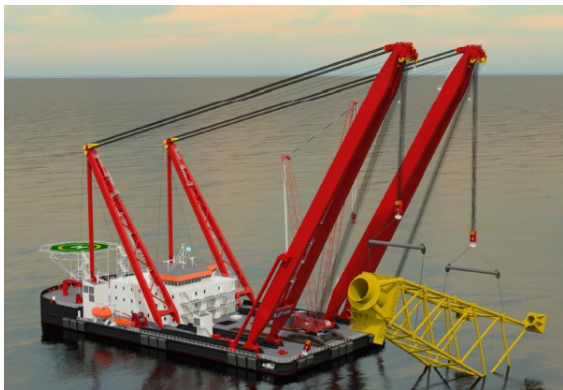
(c) Heavy lift vessel installing a jacket 10
