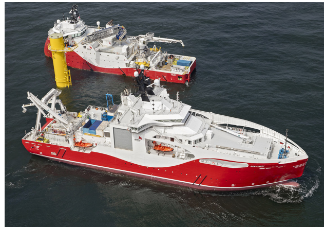
(b) Cable laying vessel and the support vessel (top) [W28]
