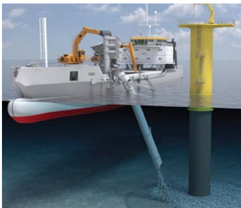
(e) Fall pipe vessel [W4]
