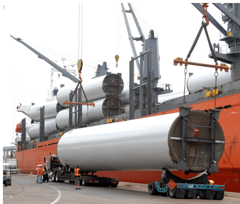
Figure 8.3: Tower component transport at San Diego USA, image by Wikimedia
