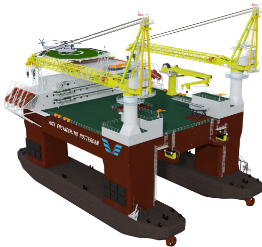
(a) Self-propelled semi-submersible [W19]
