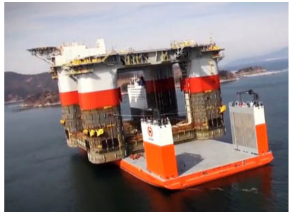
(b) Rectangular shaped semi-submersible structure transported by the Dockwise (semi-submersible vessel) in Isola del Giglio (Italy) [W22]
