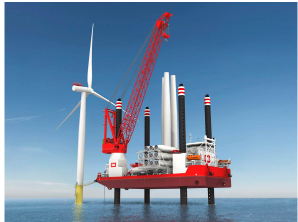
(b) Turbine installation by jack up barge 10
