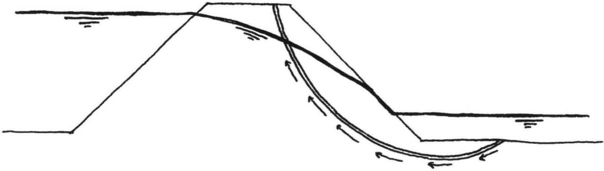
Fig.8.15 Macro-instability of inner slope of river dike at the end of extreme high water period
