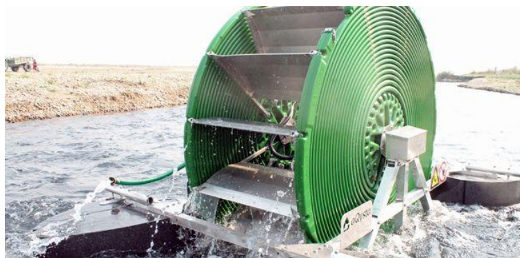
Figure 3 - Floating version of the Barsha Pump
