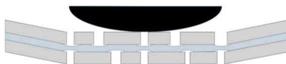
Fig. 7 Localised regions of interlayer stretching as a result of glass substrate fracture during impact testing Elziere adapted from Nourry (Elzière 2016; Nourry 2006).
