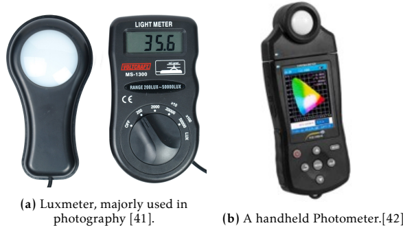
Figure 2.12: Various types of photometric devices.
