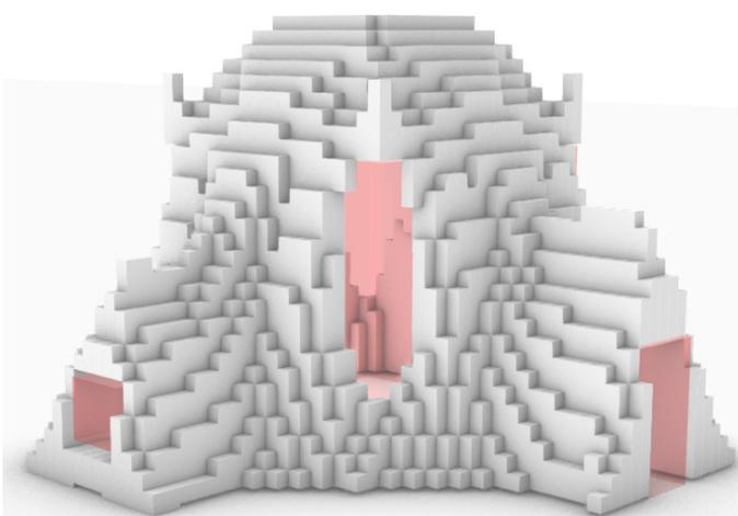
**Figure 75:** A void with door and window under selfweight
