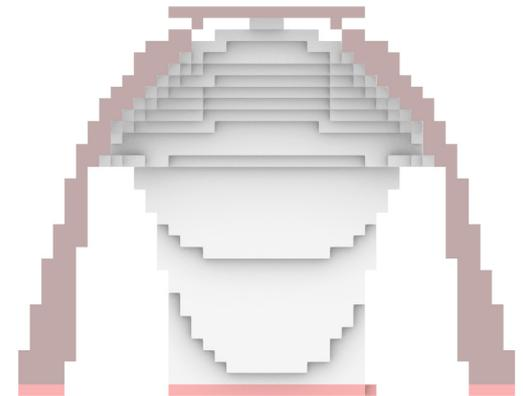
**Figure 77:** Section of the larger generated dome
