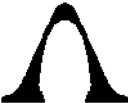
Figure 62: Shape under selfweight and extra forces
