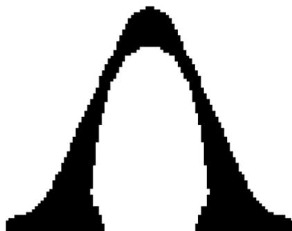
Figure 101: Arch under selfweight and snowload
