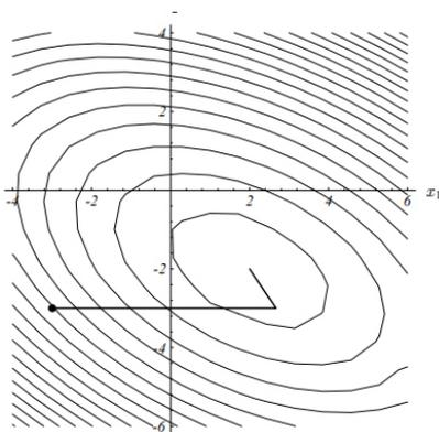
Figure 96 Conjugate gradient solver
