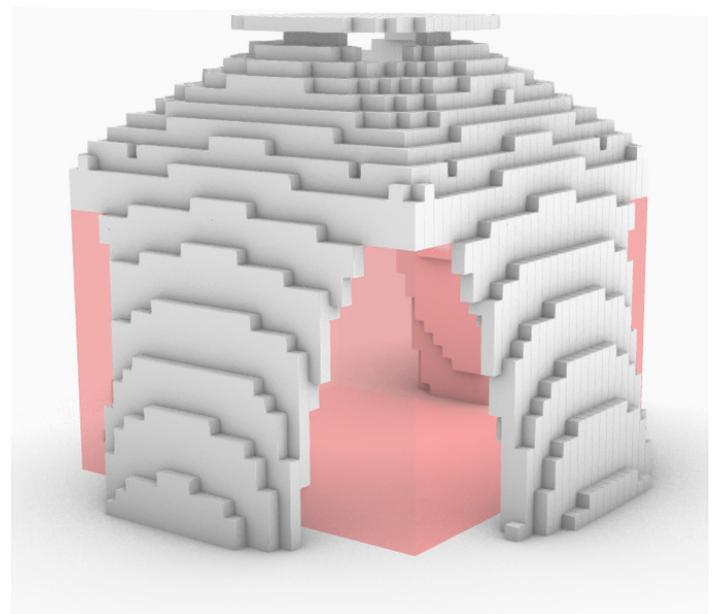
**Figure 79:** Perspective of the dome, showing the columns parallel to the void
