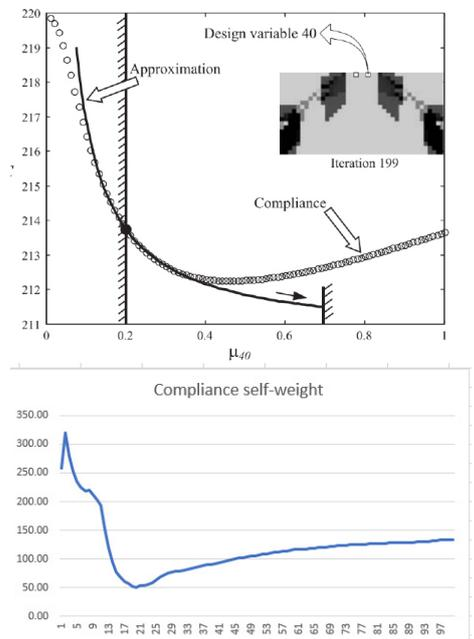
Figure 51: Selfweight over iterations
