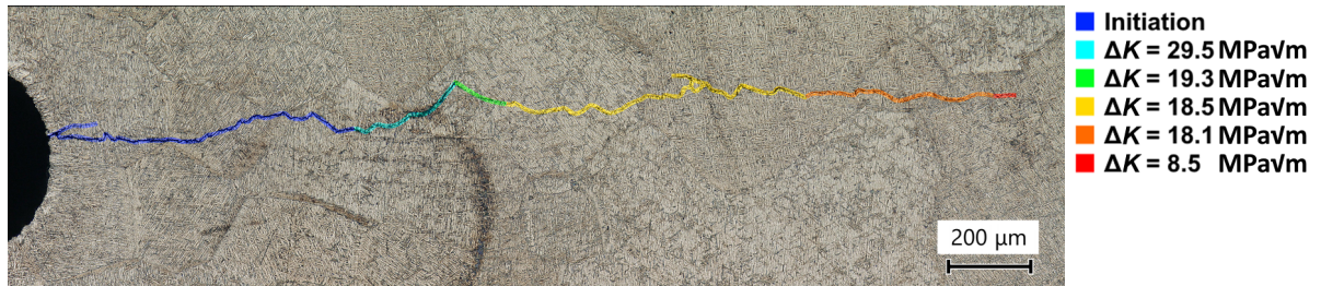
Figure 4.8: Overview of the crack path and the accompanying stress intensity range of crack 1 out of 4 on sample 1, tested at an R -ratio of 0.1
