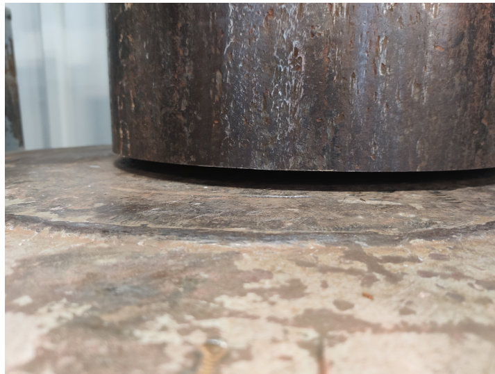
Figure 4.7: Example of pipe surface suspended from the table that provides the slip force.
