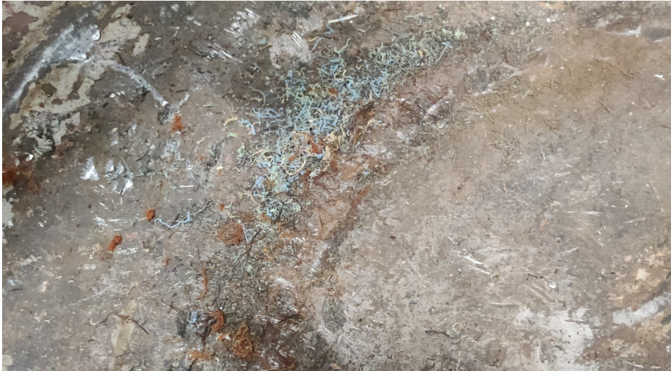
Figure 4.33: Aftermath of testing on the sandblasted 12" bare steel pipe.
