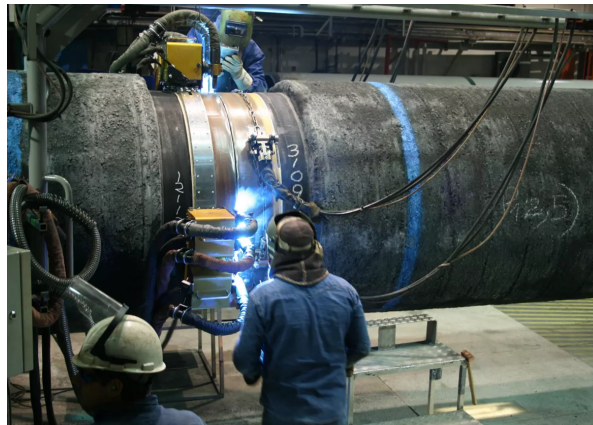
Figure 1.2: Example of a welding station on an S-lay type pipe-laying vessel from Allseas.
