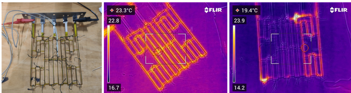
Figure 5.12: Last test of heating wireframes. On the left is the test setup, the intended result in the middle, and a short circuit on the right.
