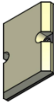
Figure 2.31: 3D representation of the current tensioner pad geometry
