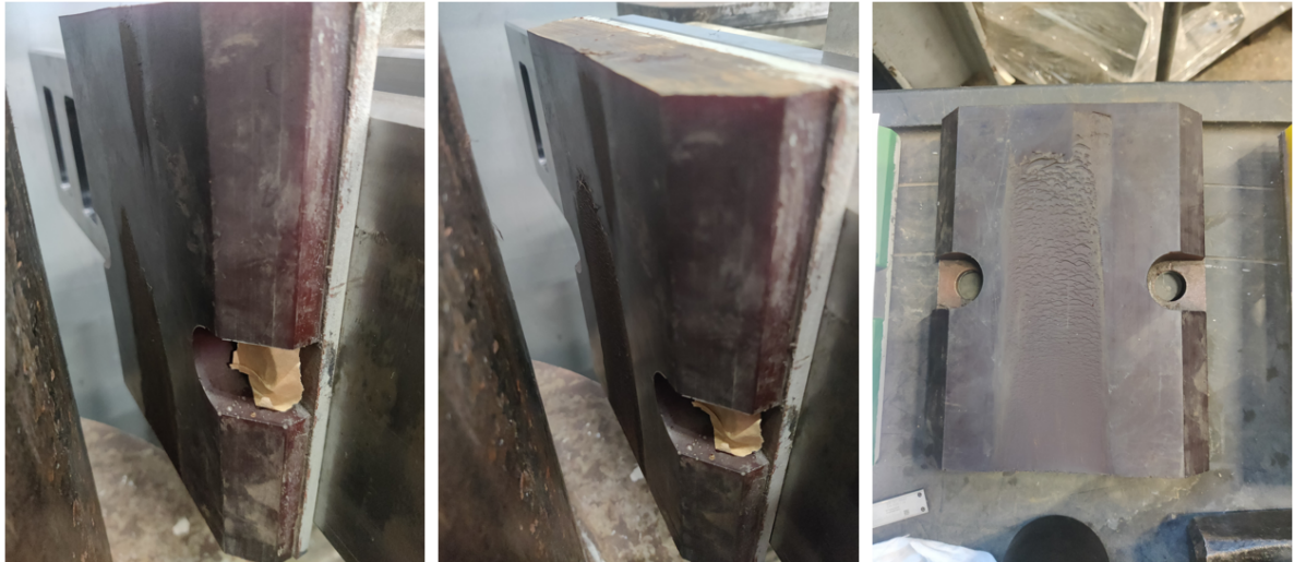
Figure 4.18: Photo's of brown 93A Shore pad damage, left photo halfway through the test sequence, middle one after roughly three-quarters of the tests and right photo after the test.
