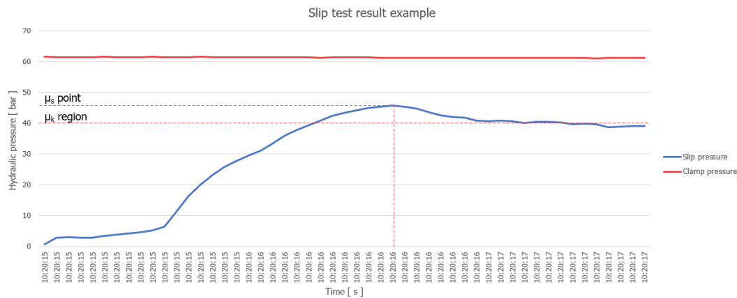
Figure 2.12: Slip test example to find the static coefficient of friction.
