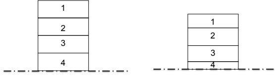
Figure 3.3: Plies with the same physical thickness and different density value.
