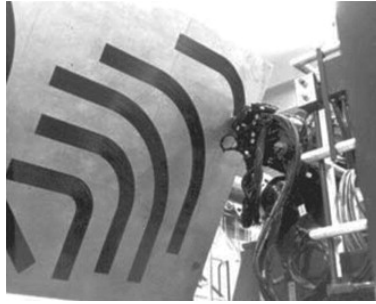
Figure 1.6: Example of fibres steered using different turning radii [16] .
