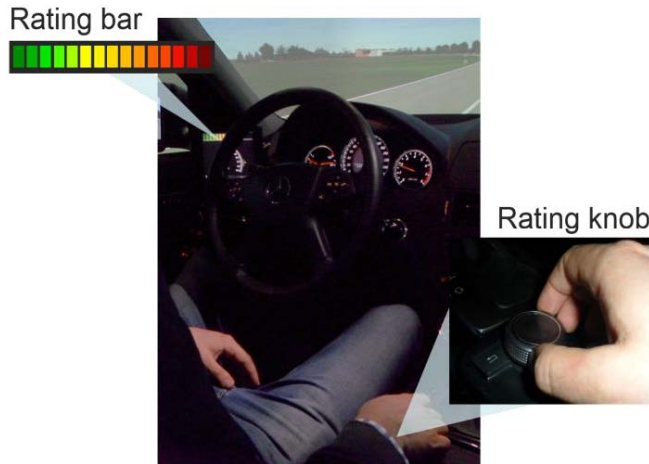
Figure 3.2: Location of rating bar and rating knob in the car cabin. The rating bar has 15 coloured marks, where green/red marks indicated low/high perceived mismatch.
