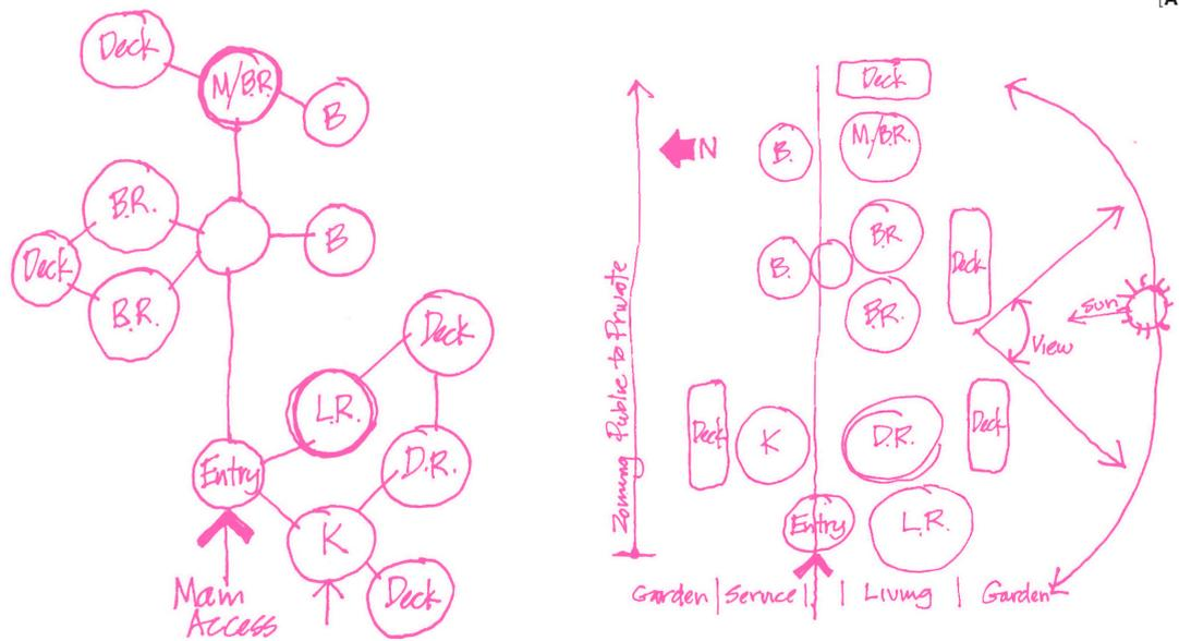
Site conditions and context are the added attributes while moulding the design in its bubble diagram phase.
