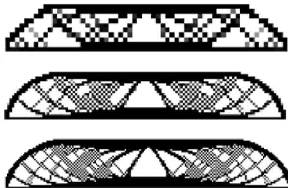
Figure 3.35: topology optimization results for different mesh sizes without using any filtering (Talischi et al., 2008)
