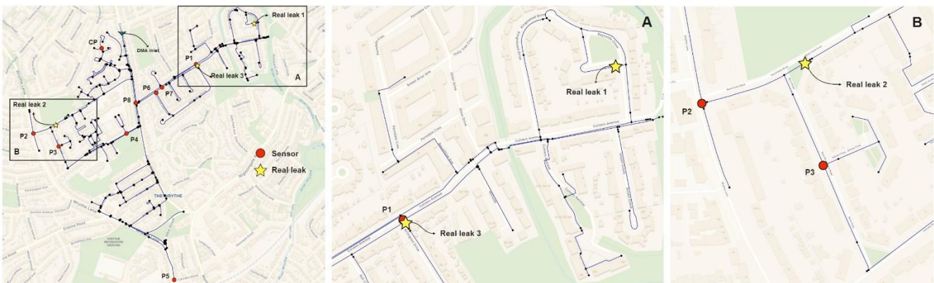
Figure 22. The network layout of DMA10 and the location of three fire hydrant leaks.
