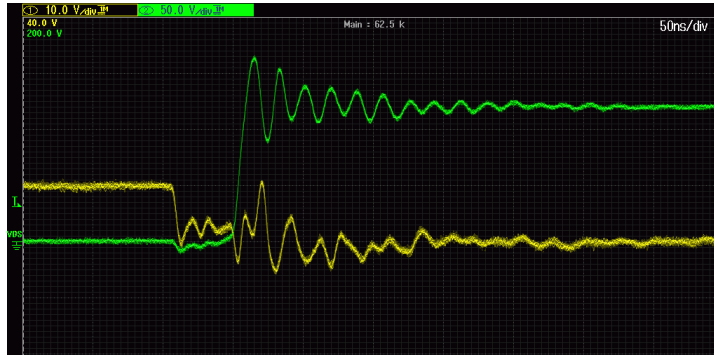
Figure 7.4: Turn-off of IRFSL4620, V_{gs} = 10V , V_{in} = 60V , R_{gate} = 5\Omega
