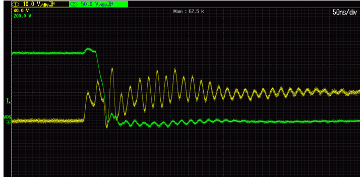
Figure 7.5: Turn-on of STF20NF20, V_{gs} = 10V , V_{in} = 60V , R_{gate} = 5\Omega
