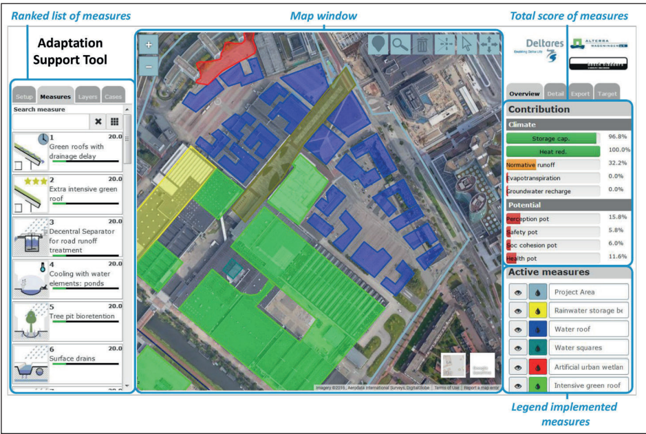
Figure 10. Adaptation Support Tool interface with three panels. The left panel includes the project set-up, the list of measures from the tool’s library, and additional layers. The map window is where measures are implemented from the list. The right panel includes the quantitative indicators of the costs and effectiveness of the applied measures, detailed impacts per measure and the adaptation targets.
