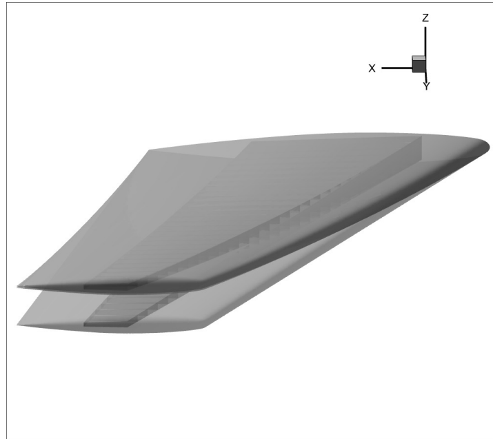
Figure 5.13: Deformed fluid- and structural meshes before and after one FSI dynamic mesh iteration.
