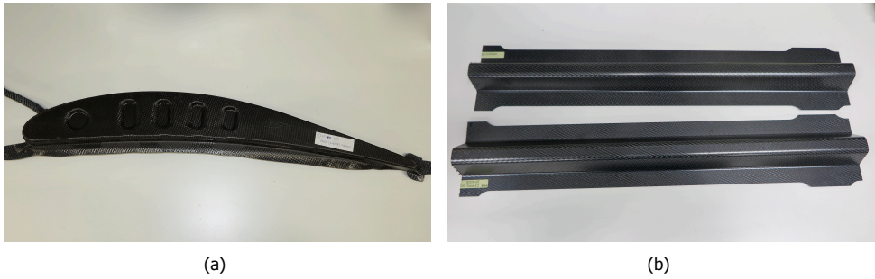
Figure 1.2: Examples of press formed aerospace parts. (a) CF/PPS rib, and (b) CF/PPS omega stiffeners.
