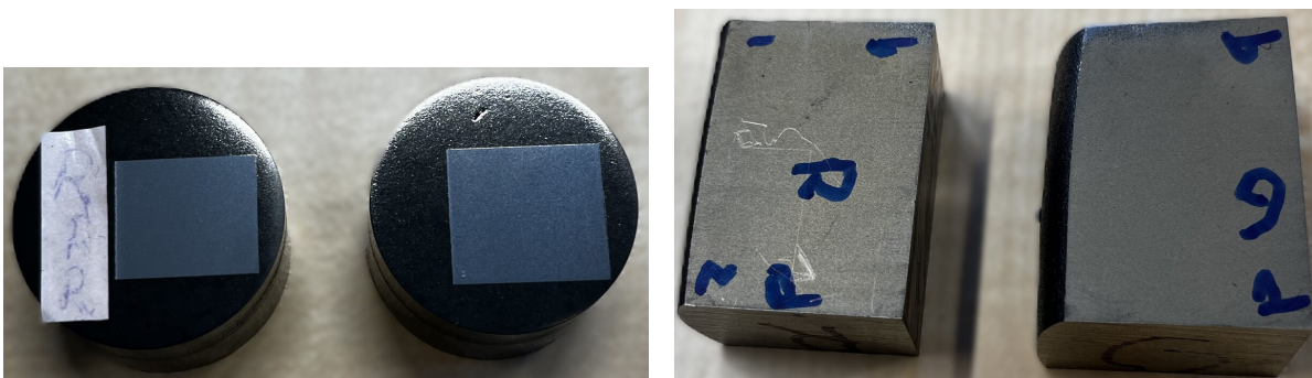
(a) SEM samples, Reference is on the left, Gasloos on the right. Cross-sections were cut so that the microstructure is viewed in the rolling direction. The left edge of the sample is the surface edge of the trailing arm.
