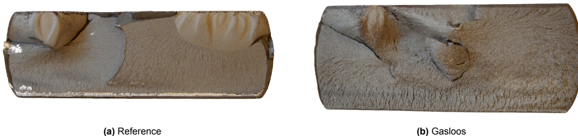
Figure 5.1: Overview of the fracture surfaces of the reference and gasloos trailing arms
