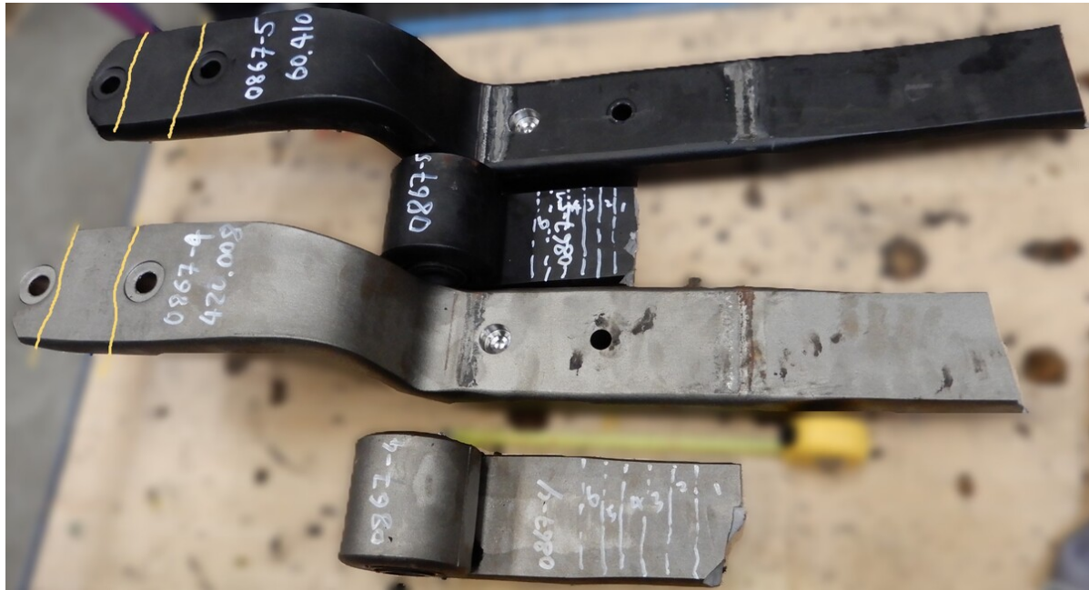
Figure 4.1: Trailing arms after bending fatigue testing. Fracture surfaces were cut from the right end, extra sections of material were cut from the left end indicated with yellow lines.
