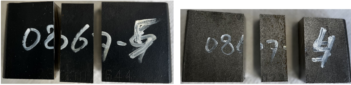
(a) Section from Reference trailing arm, with coating. Left part was used for XRD, sample for SEM was cut from middle part.
