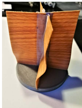
(d) Wet, deformed state, front view. Notice the wrinkling of the outer edges of the shell.
