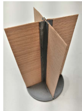
(c) Dry, undeformed state, front view. The PLA brackets are printed directly on the PLA base.
