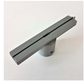
(b) Bottom part constraining the veneer and connecting the HRA to the torsion machine.
