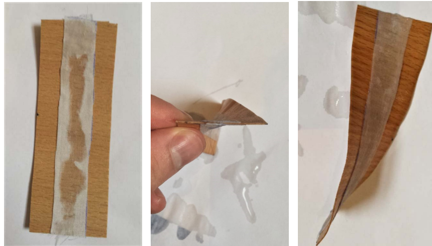
(a) Dry, undeformed state, front view. The cloth was applied with glue. It completely soaks through the cloth at some locations.
