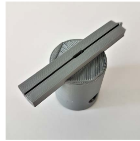
(a) Top part constraining the veneer and connecting the HRA to the torsion machine.
