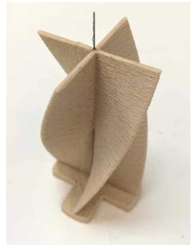
(c) 3D-printed geometry with initial twist in dry, undeformed state, front view.
