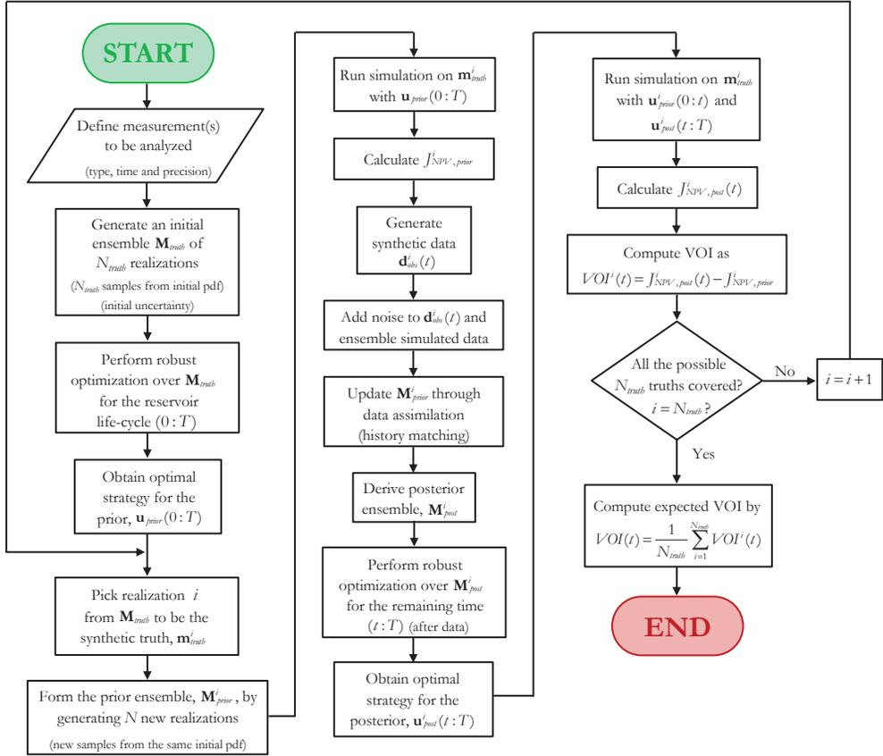
Figure 2.11: Accelerated procedure to compute the expected VOI.
