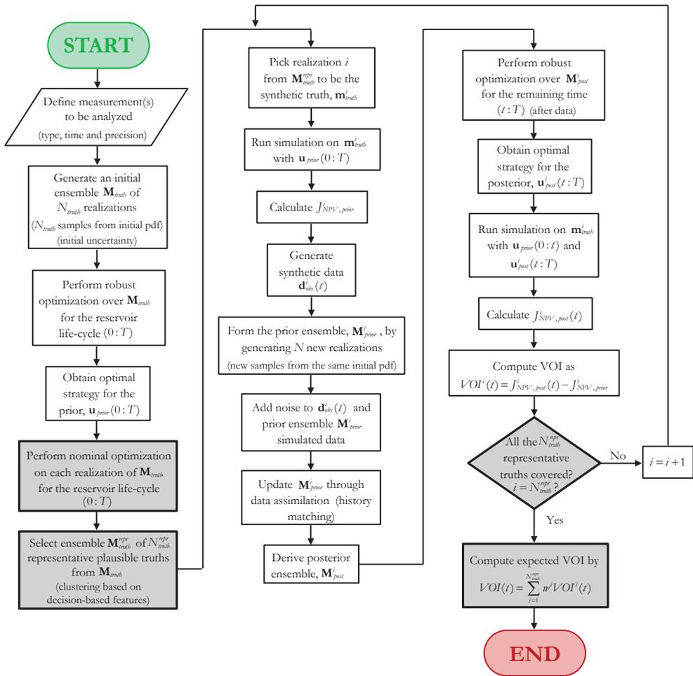
Figure 4.5: Workflow to compute the expected VOI for a single observation time using representative plausible truths and full ensembles for robust optimization and history matching. The main modifications in the workflow with respect to the original procedure (Chapter 2) are highlighted in grey bold boxes.
