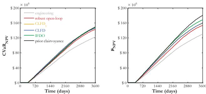
Figure 6.10: Results for the Bean model: CVaR<sub>25</sub> (left) and mean (right) of NPV for the different cases.
