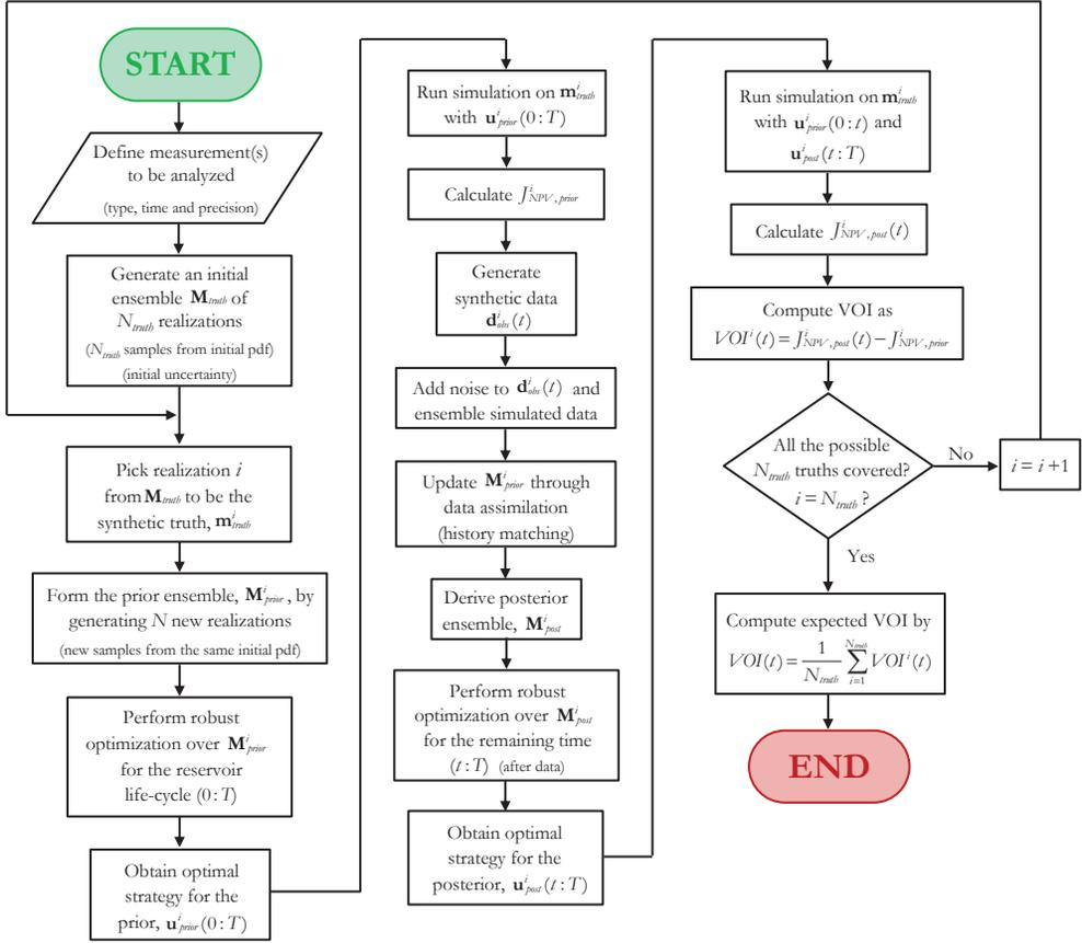
Figure 2.2: Complete workflow to compute the expected VOI.
