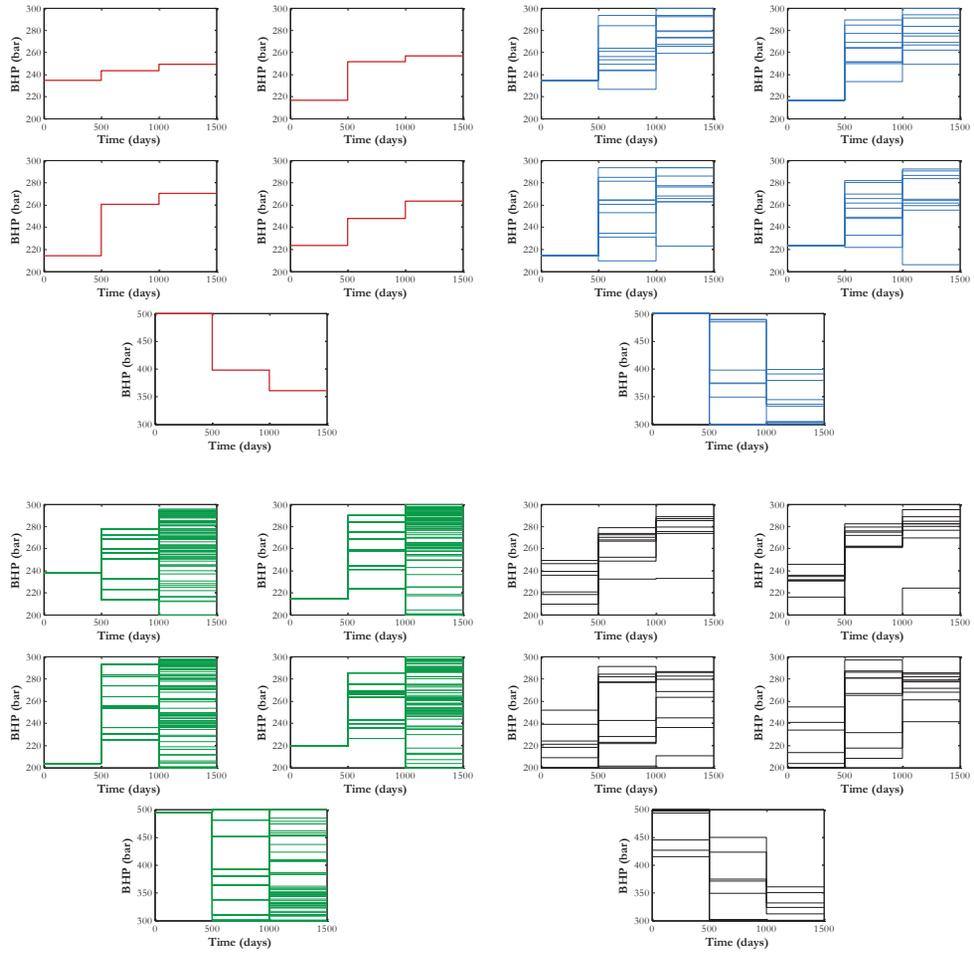
Figure 5.11: Optimal production strategies for the plausible truths considered (2D five-spot model with  $M = 3$  control time intervals): optimized under prior uncertainty (top left); obtained through CLRM with additional production measurements (top right); determined by the IPO approach with future production measurements (bottom left); optimized under the assumption of clairvoyance available at  $t = 0$  (bottom right).
