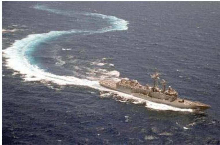
Fig. 1. A typical Zig-Zag ship maneuver in a seaway. Source: Cooperative Research Ships, Wageningen, The Netherlands.
