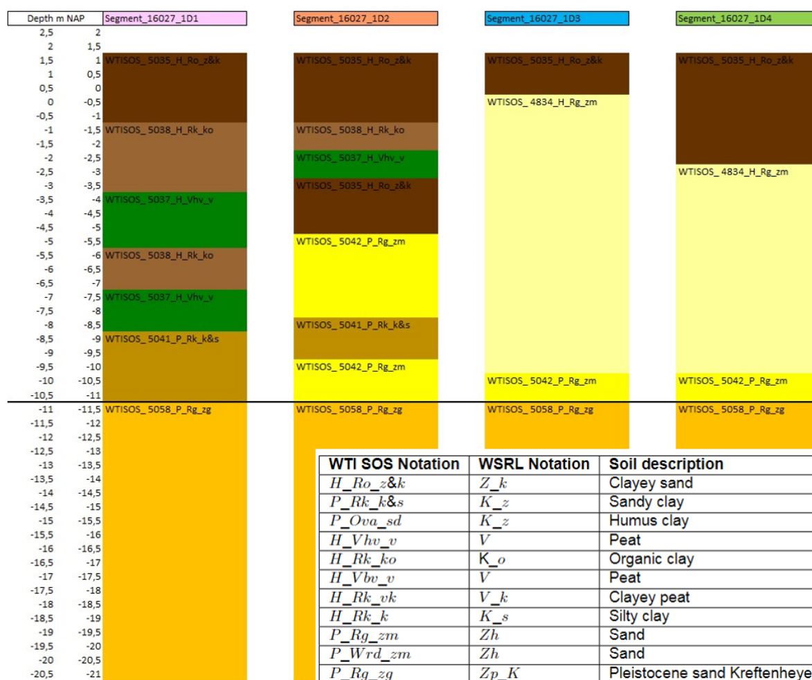
Figure 4.2: WBI Soil scenarios for Kortenhoevendijk dike trajectory, extracted from D-Soil Model (Deltares, 2017)
