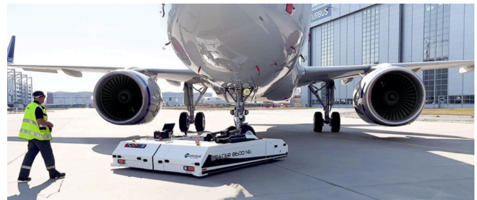
Figure 8. Trained Mototok driver performing a pushback (Mototok, 2025)
