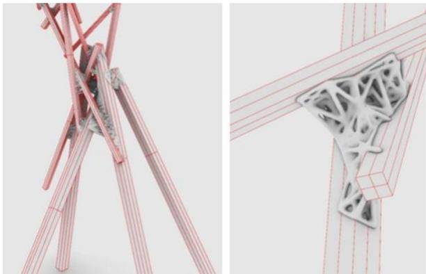
Figure 2. Optimised structural node for metal printing
