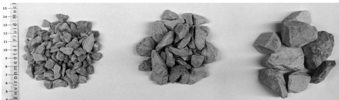
Figure B1 Filter materials. Left: Yellow Sun 8-11. Middle: Yellow Sun 10-20. Right: Yellow Sun 20-40
