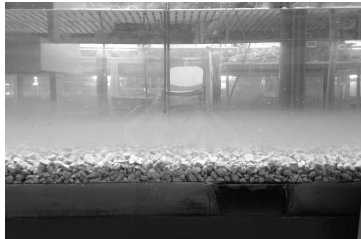
Figure C4 Dirt of the stones above the filter layer
