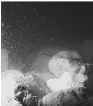
Figure 5-2 winnowing through the filter (test 6 T=2.5s H=0.08m)
