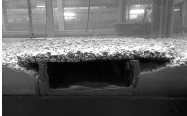
Figure 5-4 scour hole next to the tray (test 1, after a long duration test of 20 hour)
