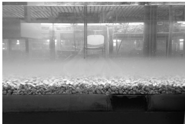
Figure 5-3 Dirt from the filter clouding the water (test 4)
