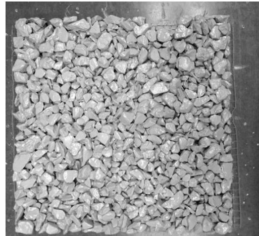
Figure 4-2 fabricated filter slab.
