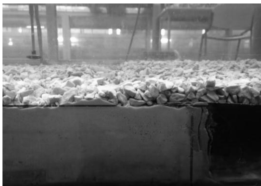
Figure C2 Scour holes after the 20 hour test ( T=2.0\text{s} H=0.12\text{m} )
