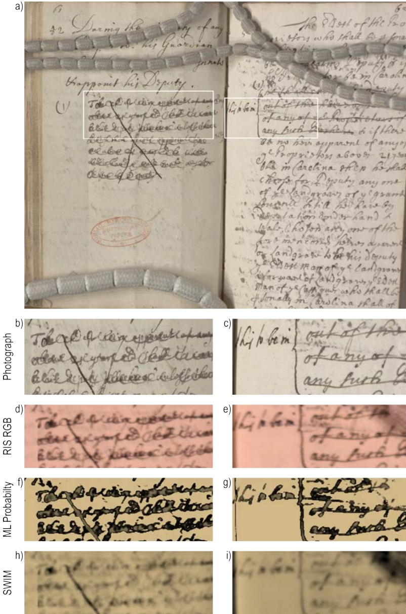
Figure 3.3.: a) Photograph of the Locke Constitution (PRO 30/24/47/3), with the two example areas marked. b-c) Detail photograph of the two example areas. d-e) RGB derived from the RIS data, produced using the XYZ method in DataHandlerP[22] f-g) Probability maps output by the classifier shown in a special manuscript colourmap for the Text Ink class. h-i) SWIM for the Text Ink class shown in a special manuscript colourmap.
