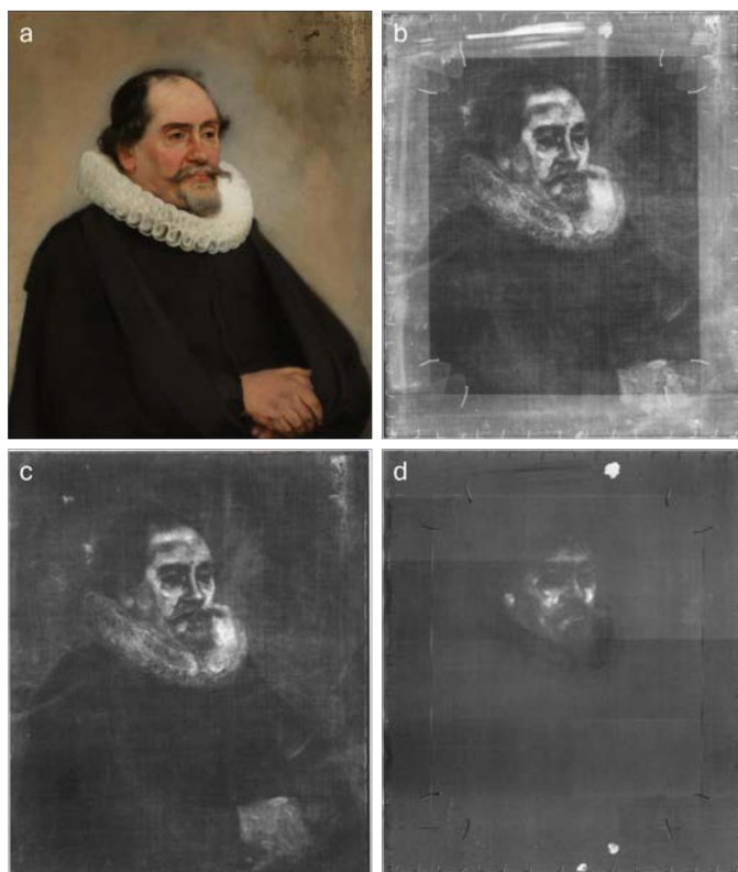
Figure 1.3.: Carel Fabritius, Abraham de Potter (1592-1650). Amsterdam Silk Merchant , 1649, oil on canvas, h 68.5 cm x w 57 cm, Rijksmuseum, Amsterdam (inventory nr. SK-A-1591).[13] (a) Visible light photograph. (b) Conventional XRR, showing the difference in X-ray absorption between the paints as well as the wooden stretcher. (c) K-edge absorption image for Pb (low energy 87.3 keV, high energy 88.7 keV) showing the lead white distribution. (d) K-edge absorption image for Hg (low energy 82.4 keV, high energy 83.8 keV) showing the vermilion distribution. Modified from [12].
