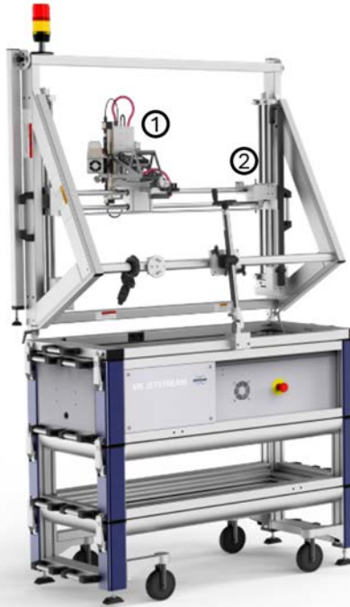
Figure 1.8.: The most widely adopted MA-XRF is the Bruker M6 Jetstream. Highlighted are (1) the scan head which includes the X-ray source, polycapillary lens and two SDD X-ray detectors; and (2) the Cartesian coordinate robot positioning system.
