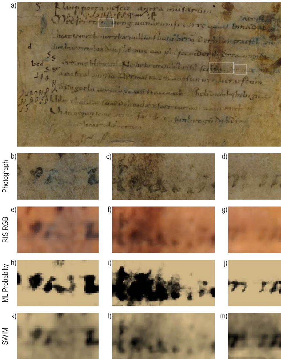
Figure 3.1.: a) Photograph of the Leiden Riddle, with the three interest areas marked. b-d) Detail photograph of the three interest areas. e-g) RGB derived from the RIS data, produced using the XYZ method in DataHandlerP.[22] h-j) Probability maps output by the classifier shown in a special manuscript colourmap for the Riddle Ink class. k-m) SWIM for the Riddle Ink class shown in a special manuscript colourmap.
