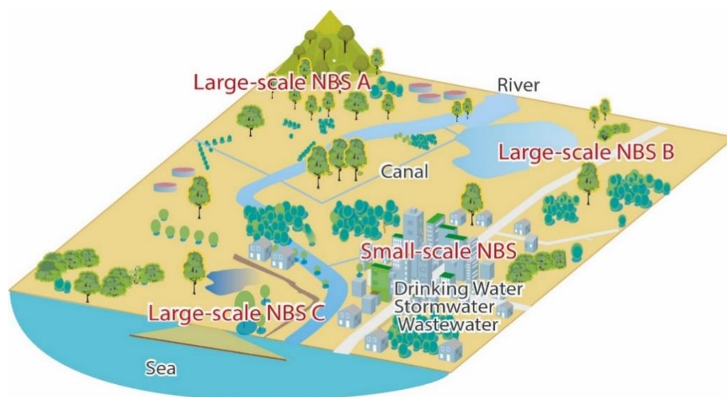
Figure 1.2. Illustration of large- and small-scale Nature-Based-Solutions (NBS); Large-scale NBS A illustrates NBS in mountainous regions (e.g., afforestation, slope stabilization, etc.), Large-scale NBS B illustrates NBS along river corridors (e.g., widening river, retention basins, etc.) and Large-scale NBS C illustrates NBS in coastal regions (e.g., sand dunes, protection dikes/walls, etc.); Typical examples of Small-scale NBS are green roofs, green walls, rain gardens, swales, bio-retention, etc.
