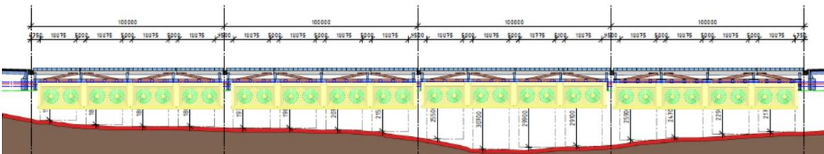
Figure D.12: Surface area facing perpendicular flow;  $\alpha = 0$  (Vos, 2017)
