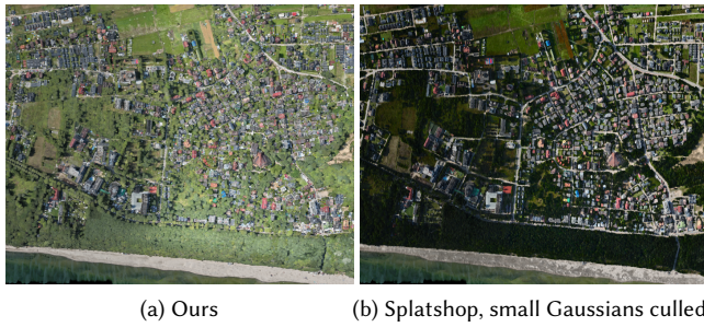
Fig. 9. The optional culling of small Gaussians in Splatshop is beneficial to its scalability but introduces strong artifacts. In this distant view, most Gaussians are small and thus get culled. Only 8.2 M out of the 106 M Gaussians in the scene get rendered. Without culling of small Gaussians, Splatshop cannot render this scene. Our method splats points for every single Gaussian with the right probability.
