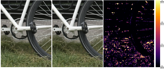
Fig. 7. A comparison between K = 1 (left) and K = 4 (middle), both with converged images and 2 \times 2 supersampling. To the right, we show the per-pixel RMSE between these two images. The full 1920 \times 1080 frames take 13.3 ms and 9.7 ms to render, respectively.
