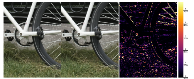
Fig. 6. Converged results of our method (left), 3DGS (middle) and per-pixel RMSEs between the two images (right). Differences in aliasing cause slight bias in high-frequency regions.
